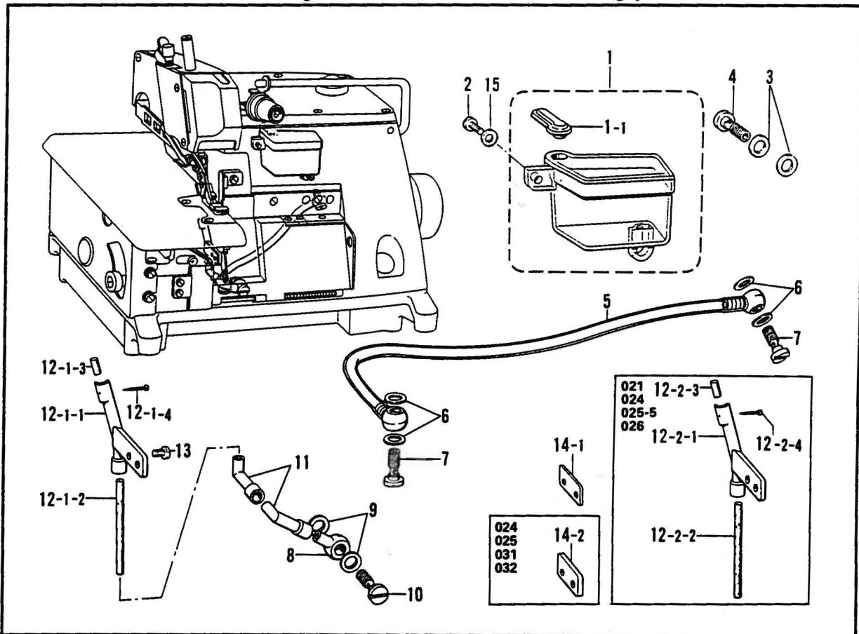
B. 駆動軸関係/Crank shaft mechanism/Kurbelwelle/
