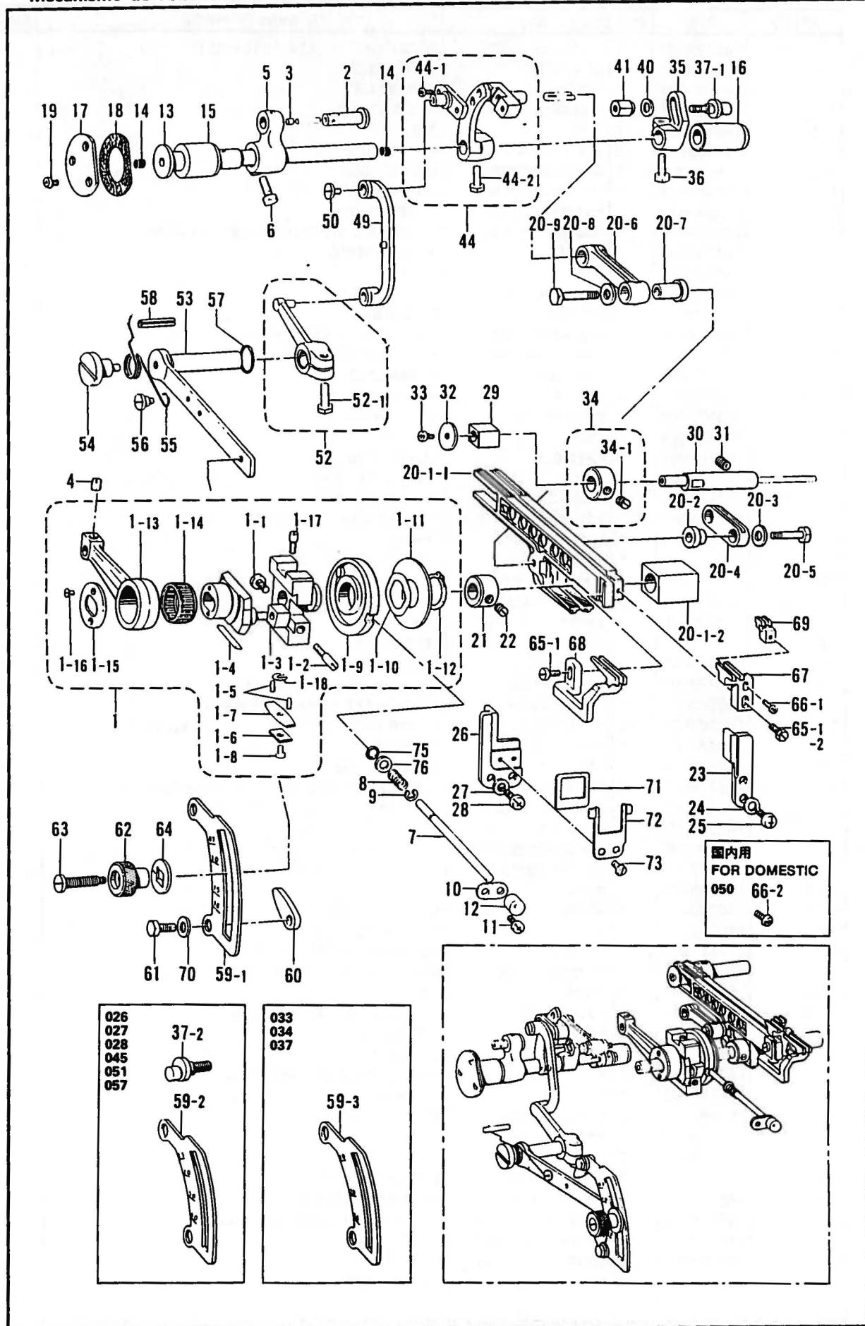
F. 送り関係/Feed mechanism/Transportvorrichtung/
